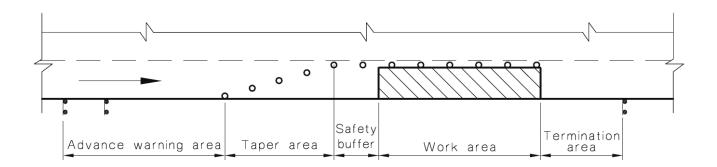
Advance Warning Area: The area before the work zone where signs and devices should be placed to warn road users that work is taking place and that there will be workers on or near the roadway.
