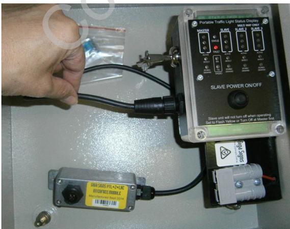
6. Connect the PTL-2-LHC Cable to the Interface Module.
