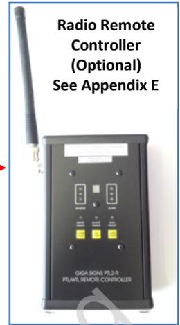
With the lamps in Flash Yellow condition, press “MANUAL” on the Hand Controller to enter Manual Mode.
