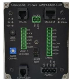
NB: When batteries are flat, the units will enter into Flash Yellow mode automatically.
