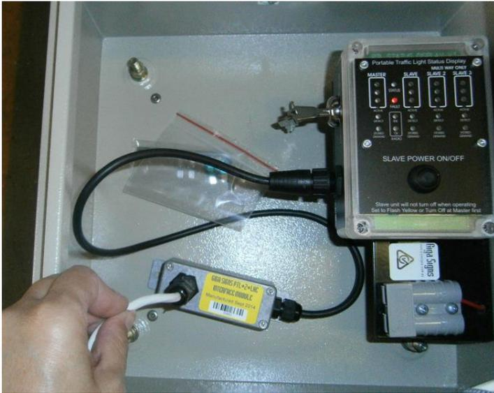
7. Plug the opposite end of the PTL-2-LHC Cable into the PTL-2-LHC. The PTL2 unit is now ready to be controlled by the PTL2 LHC.
