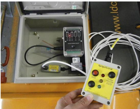
8. Turn the traffic Lights ON by holding down the “Flash Yellow” button for 4 seconds. The unit will display flash yellow.
