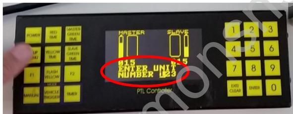
6. Turn the SLAVE unit off by pressing the Power button on the hand controller. Repeat steps 3 to 5 with the MASTER unit.
