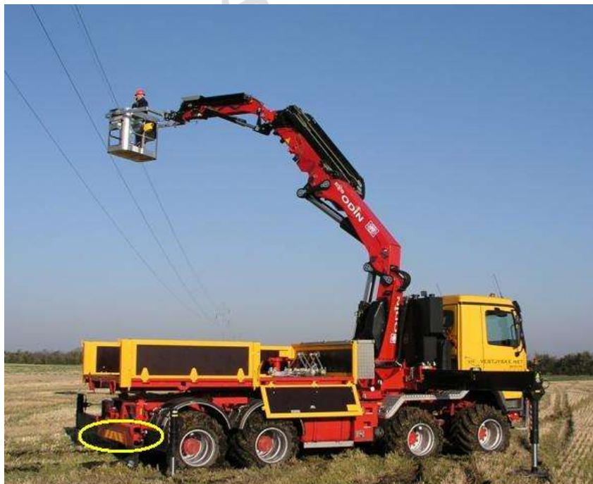
Fig. 7. A safe lifting method for personnel: An Elevated Work Platform.
